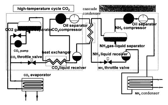
Unlike conventional low-temperature refrigerants, CO<sub>2</sub> has the characteristics of low evaporating temperature and high operating pressures. This presents challenges for the development of CO<sub>2</sub> low temperature systems:
